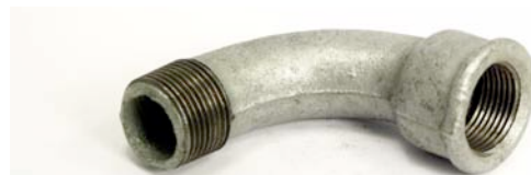
BEND STREET MALE / FEMALE Malleable Cast Iron THREADED PT GALVANIZED Nr 1 90 degr.
