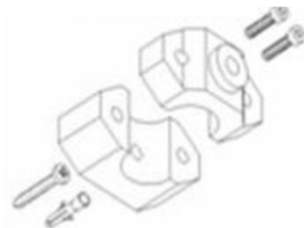
Important to install the bracket to protect hose and connector
