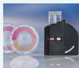
Testing of free and total chlorine
