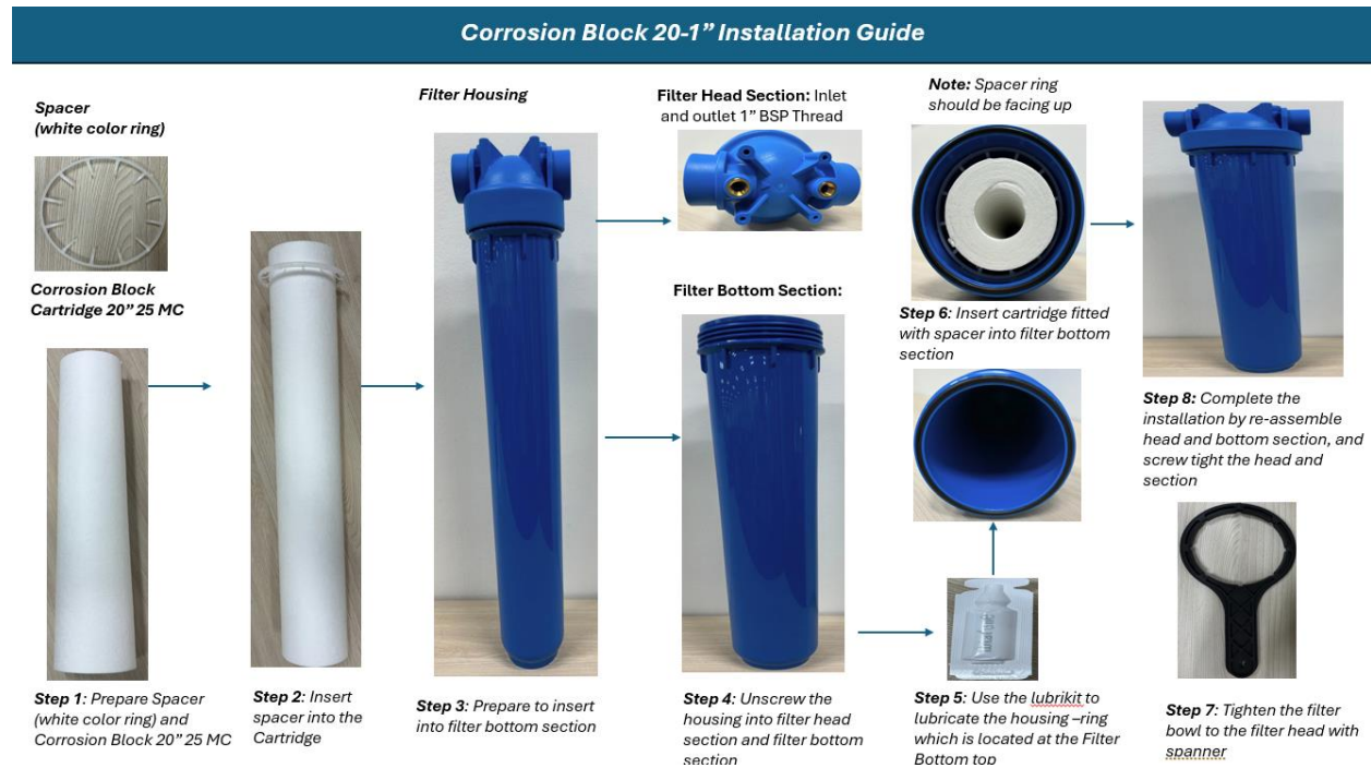
Pic 5: Installation Guide For Corrosion Block 20-1"
